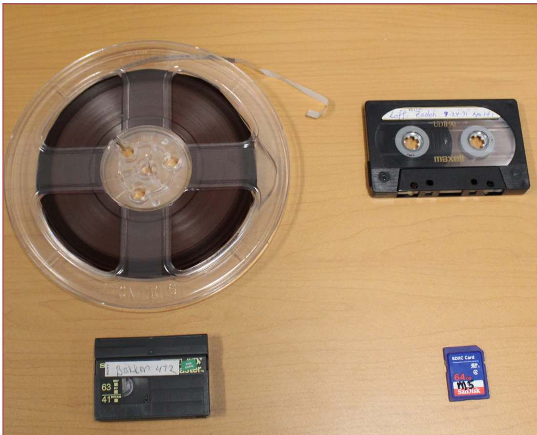
Evolution of the IEEE History Center's physical media: Top row: Oral history #001 on reel-to-reel tape, oral history #112 on cassette tape; bottom row: Oral history #472 on DV tape, SD card used in current oral history camera
